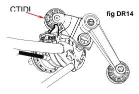
the rear frame inverted) the chain as per fig AR3. For a derailleur bike, the chain and the fixed idler on the chain-tensioner-base, CTIDLB, have to lie between the "uprights" of the chain-pusher-plate: so, with the LH trigger up and the chain-tensioner inclined slightly outwards as in fig DR14 (chain not shown in this figure), feed the idler CTIDLB between these uprights, and then feed the chain-tensioner base onto the rear axle plate till it abuts squarely.
