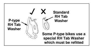
The kit is used as follows: Insert the Bolt through the Bush then the RH tab-washer and into the axle from the RH side. Ensure the LH tab-washer and wire-form is in place and screw-on the Nut with the knurled detail outermost and tighten to 8Nm maximum keeping the wheel central between the forks.
